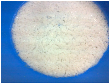
Figure 2. Microencapsulation phase change Material (MEPCM)
