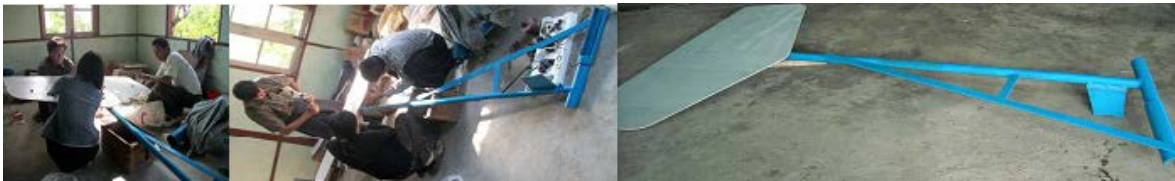
Figure 6. Tail vane bolted to the tail boom
