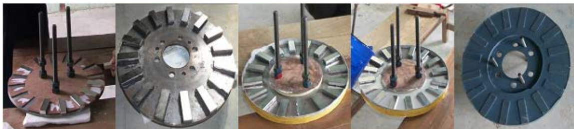
Figure 1. Construction of rotor discs
