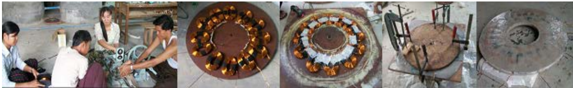
Figure 2. Stator coils casting from the mould
