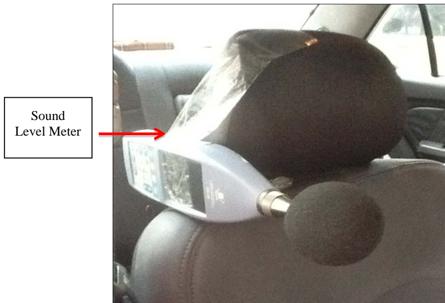
Figure 2. Location of the sound level meter (SLM) at the driver's ear position
