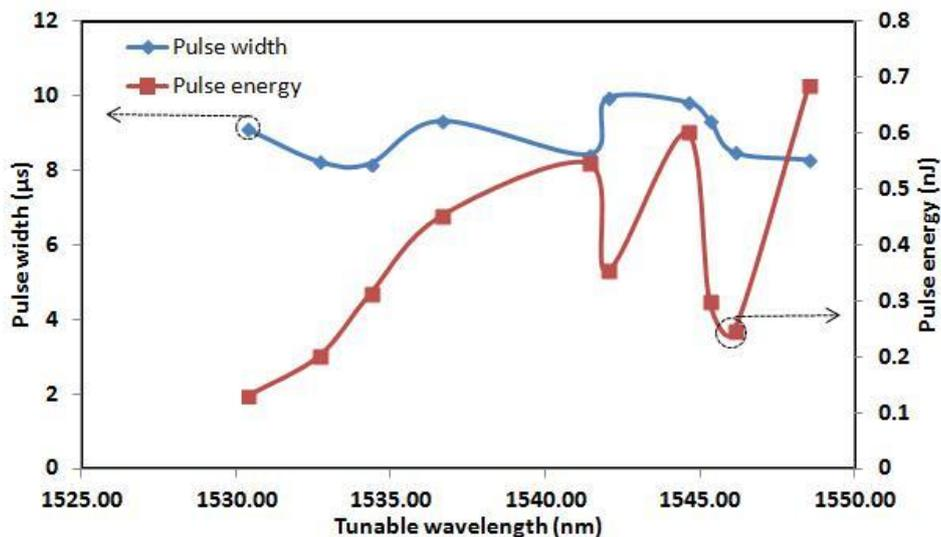
Figure 7. Pulse width and energy versus tunable wavelength
