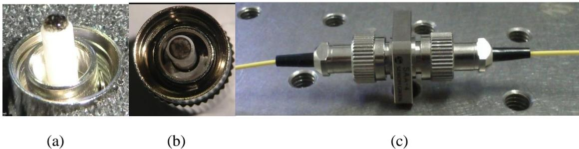
Figure 1. (a) Droplet of SWCNT-PEO (b) Thin layer after left in room temperature for 24 hours (c) Integration in fiber laser
