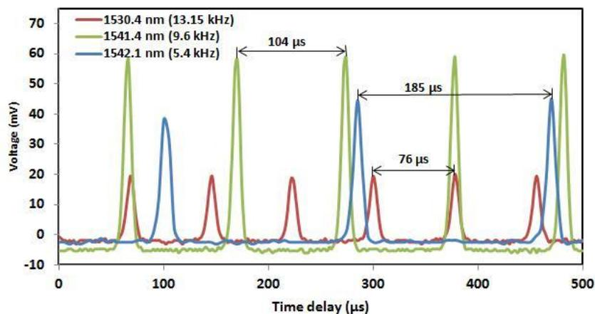
Figure 5. Train of pulses for tuneable wavelength at 1530.4 nm 1541.4 nm and 1542.1 nm
