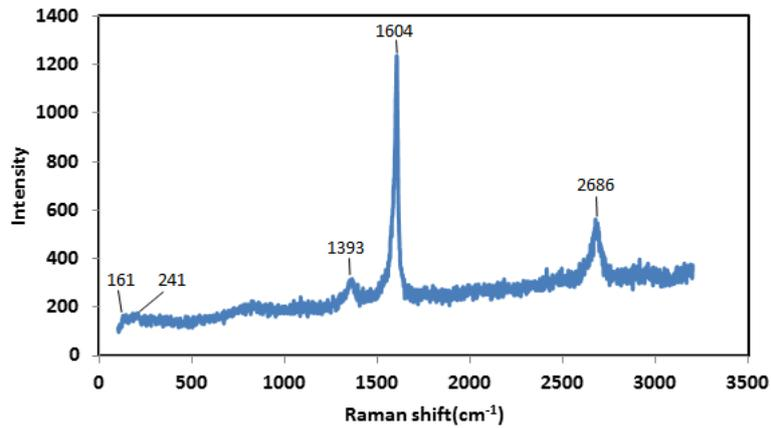
Figure 2. Raman spectrum of the SWCNT polymer composite deposited on the fiber ferrule
