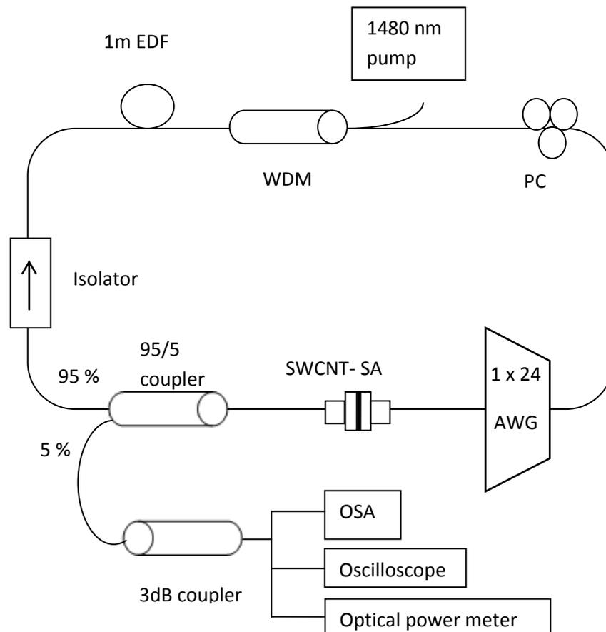
Figure 3. Experimental setup of the proposed tunable fiber laser. (PC: polarisation controller; AWG: arrayed waveguide grating; SWCNT-SA : single walled carbon nanotubes saturable Absorber; OSA: optical spectrum analyser; WDM: 1490/1550 nm wavelength division multiplexer; EDF: erbium-doped fibre)
