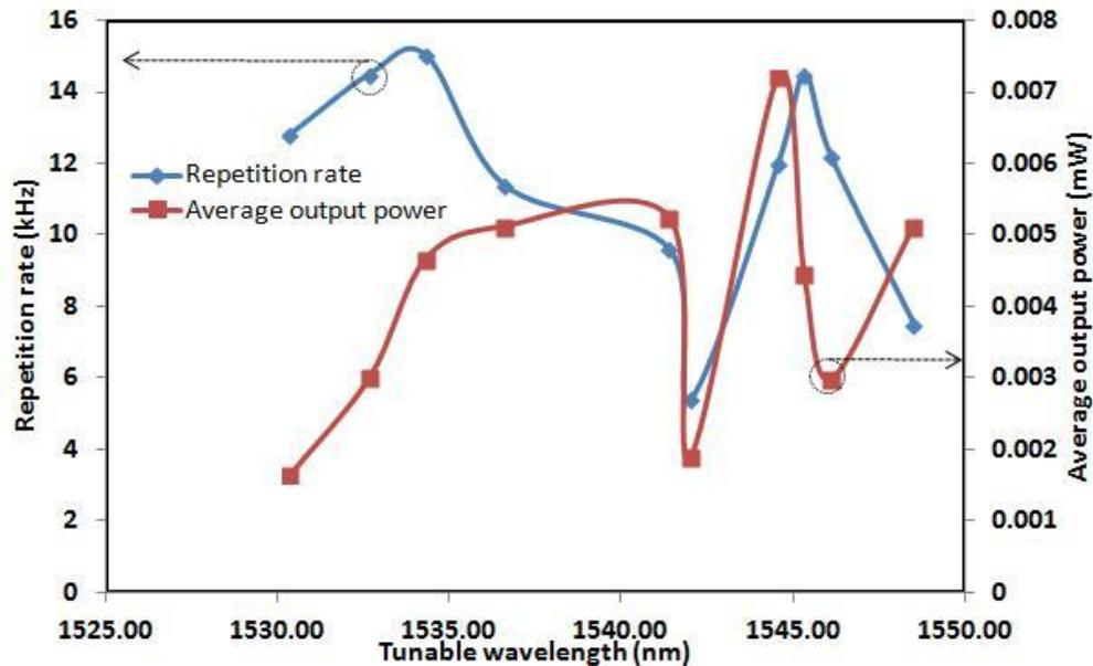
Figure 6. Pulse repetition rate and average output versus tunable wavelength
