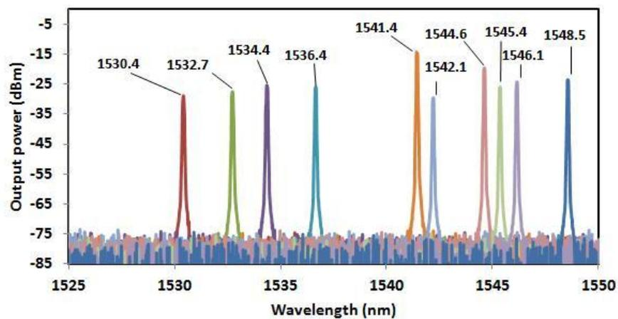
Figure 4. Tuneable wavelength fiber laser
