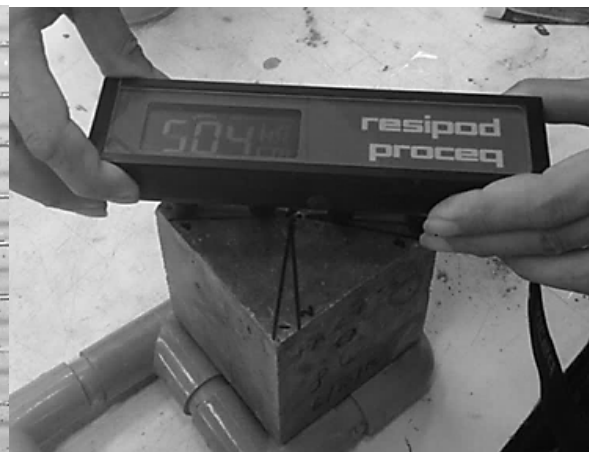
Figure 3. Measurement technique for electrical resistivity of a cubic specimen using four Wenner probe
