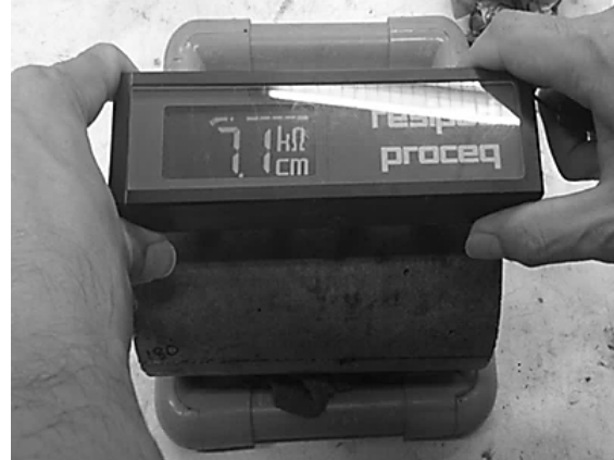
Figure. 5 Measurement technique for electrical resistivity of a cylindrical specimen using four Wenner probe
